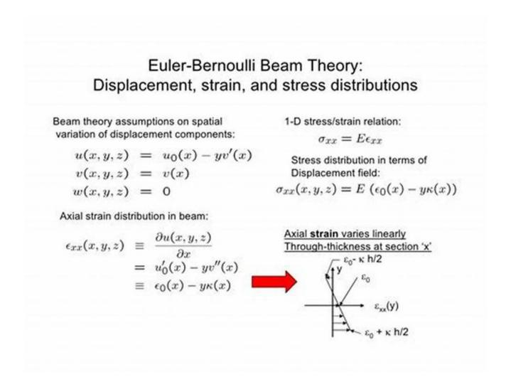
The Euler-Bernoulli equation describes the behavior of slender beams subjected to bending. It provides insights into the distribution of bending moments and deflections along the length of the beam, enabling engineers to design beams that meet specific requirements.
