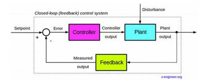
Feedback allows for self-correction, ensuring that the actual system behavior matches the desired response. By analyzing the difference between desired and actual system outputs, control systems can take corrective actions, such as adjusting control signals or initiating alarms, to maintain system integrity and performance.
